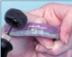
FIG. 25: SMOOTH THE ROUGH EDGES WITH AN ESSIX POLISHING BRUSH.
